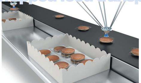
Adsorbing unstable, soft film-wrapped workpieces with high speed spider robots in the food industry require a highly adaptable pad skirt. To this end, use our FDA compliant blue vacuum pads – ZP3P Series
