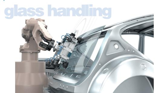
Adsorption marks must not be left on workpieces in glass handling applications. To this end, use our markfree vacuum pads – ZP2 series
